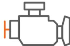
This input is designated to detect when your engine is on or off. This input will provide a display of accumulated engine hours on the Mobile and Fleet Apps. If NMEA 2000 is connected, the engine hours information from NMEA will override the ignition wire input.
